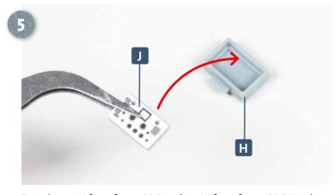
Detach part H from frame 23-2 and part J from frame 23-3. Apply some glue to the edges of J and fit inside the opening of H, as shown in the photo above.
