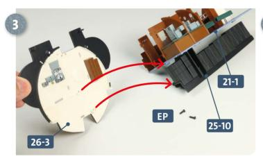
Have two EP screws ready. Take the aft bulkhead 26-3 and align its two holes so they fit over the sockets at the base of 21-1 and on the installation rail 25-10, respectively, in the positions shown by the two arrows. Take time to ensure all the tabs are correctly seated into their slots.
