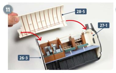
Take the deckhead panel 28-5 and fit it between the two bulkheads 26-3 and 27-1, so that the fixing holes are aligned.
