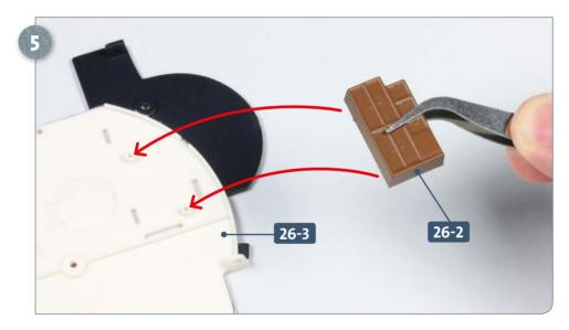
Take the lockers part **26-2**. Apply some glue to the two sockets on the back and attach it to the two pegs on the bulkhead **26-3**, as shown by the arrows.
