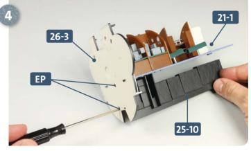
Once happy with the positioning, first add some glue to the contact points of both assemblies. Fix the bulkhead 26-3 to the deck 21-1 and the installation rail 25-10 in the position previously practised, using two EP screws, as shown.
