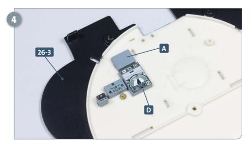
Remove part **D** from frame **26-1**, apply some glue to the two sockets on the back, and attach to the bulkhead as shown in the photo.
