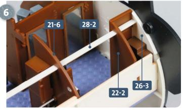
Continue to feed the pipe 28-2 through the notches in room dividers 21-6 and 22-2, until it abuts the aft bulkhead 26-3.
