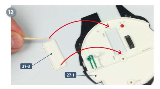
Orientate the soundproof door 27-3 as shown. Apply some glue to the two small pegs at the top and bottom of the door. It is then glued into the large opening in the bulkhead 27-1 (see arrows).
