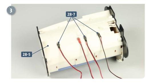
The three white LEDs 28-7 (L-1) are installed in the remaining three holes in the deckhead 28-5, as shown.
