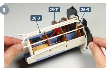
Take the pipes 28-3 and glue the narrow end into the two holes in the bulkhead 26-3. Again, the underside mount is glued to the remaining peg on the partition bulkhead 23-11 (see arrow).
