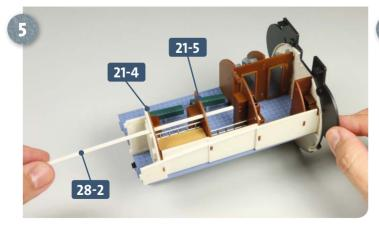
Orientate pipe 28-2 so that its smaller side faces downwards, and route it through the cut outs in the room dividers 21-4 and 21-5, as shown.
