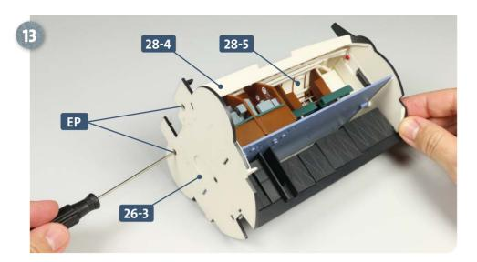
Next, secure the deckhead 28-5 to the aft bulkhead 26-3 using two EP screws, as shown in the photo.
