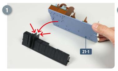
The underside of the compartment 21-1 is first fitted onto the ammunition box/battery cell assembly you built in kit 25. Add glue along the top edges as indicated by the two straight arrows.
