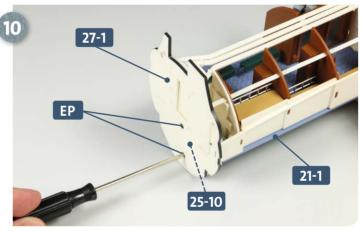
Once happy with the positioning, apply some glue to the contact points before attaching the bulkhead 27-1 to the deck 21-1 and the installation rail 25-10 using two EP screws, as shown.
