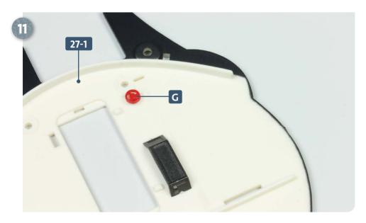
Remove the hand wheel **G** from frame **27-2**. Glue this in position at the top of the bulkhead **27-1**, as shown in the photo: the peg on the back of the wheel fits into the hole.
