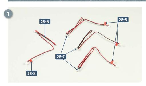
Label the three white LED cables 28-7 (these each have a black sleeve) with one of the cable lables 28-8, printed with a 'L-1'. The red LED cable 28-6 (with the red sleeve) should be marked with the 'L-2' cable label. Attach the cable labels approximately 8mm from the terminal end of the LED cables. You may wish to test the LEDs in a similar way to that described in steps 1 and 2 of kit 24.
