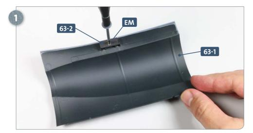
Place the hull plate **63-1** on your work surface, inside facing up. Take the metal plate **63-2**, with the countersunk side upwards, and fit it flush to the raised socket on the hull plate and fix in position using an **EM** screw, as pictured.
