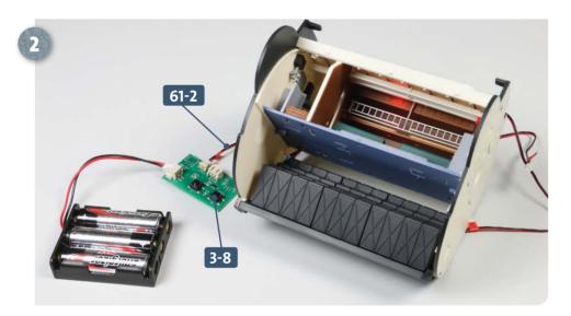
When cable **61-2** (labelled **L2**) is inserted into the test PCB **3-8** the LED should light red.
