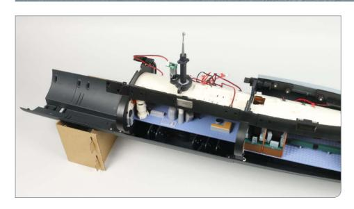
Two connectors and a magnet (fixed onto a mounting plate) have now been added to the hull assembly.
