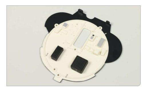
Two fuel oil collection bunkers have now been assembled and attached to the forward bulkhead of the engine compartment, along with other details.
