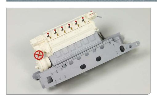
The engine is taking shape with the cylinder cover and various other details now attached to the assembly.
