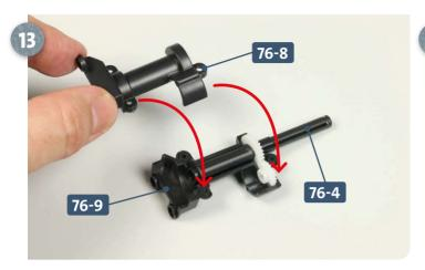
With the shaft **76-4** in place in the mount **76-9**, take the back half of the mount **76-8** and fit it onto the assembly, as indicated by the arrows.
