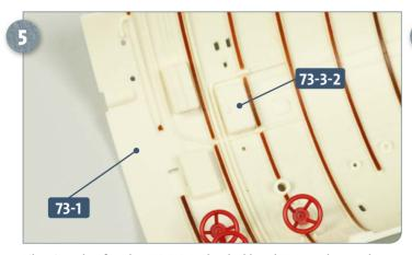
Likewise, glue fuse box 73-3-2 to the deckhead 73-1, as shown above.
