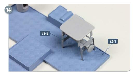
Turn the bracket **72-5** over once more. Apply some glue to the four legs and insert into the slots in the forward section of the engine room deck panels **72-1**.
