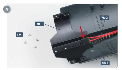
This photograph shows the connector **78-1** in place against the hull plate **48-1**. The ledge at the forward end of the connector, indicated by the arrow, is positioned over the contact wire board **78-2**, as shown. Have ready four **FM** screws.
