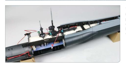
The testing of the two motors for the navigation periscope has been completed. The supplied hull section (not pictured) will be added in a later kit.
