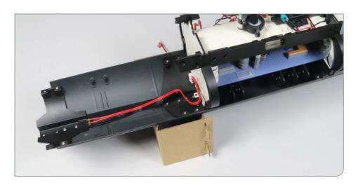
A contact circuit board and connector have now been added to the main assembly.
