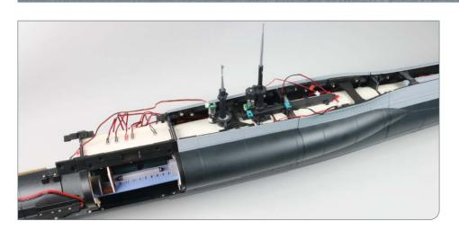
A third removable hull section has now been attached to the starboard (R) side of the U-Boat.
