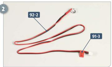
Remove the cable label 91-3 with the label L2 from the backing film, and attach it to the cable 92-2, approximately 8mm from the end with the plug.
