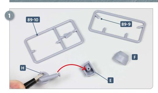
Place frames **89-9** and **89-10** on your work surface. Detach the main parts of the coupling, **E**, **F** and **H**. Apply some glue to the narrow end of **H** and glue it into the recess of part **E**, as indicated by the arrow.
