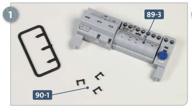
Place the main switchboard assembly **89-3**, from the previous kit, on your work surface. Taking frame **90-1**, detach the three levers.
