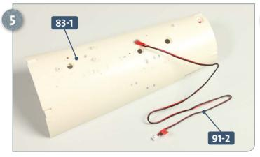
Insert the red LED **91-2** into the hole in the deckhead of the electric motor room **83-1**, as shown.
