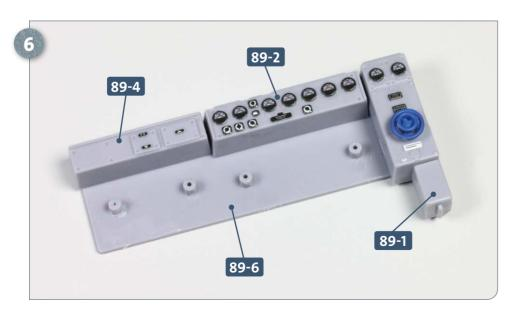
Glue the voltmeter and ammeter **89-2** and the field regulator **89-1** to the rear panel **89-6** next to the fusebox, as pictured, left.
