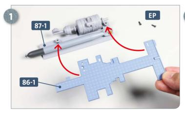
Have ready the base plate **87-1** and two EP screws. Take deck plate **86-1** and place its two mounts on the holes in the base plate, as indicated by the two arrows.
