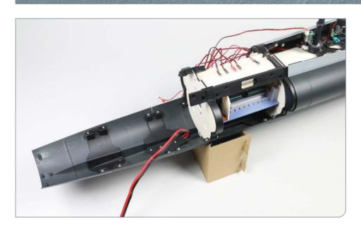
A connector and an additional hull section have now been added to the aft end of the main assembly.
