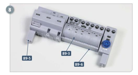
Glue the switchboard **89-3** to the rear panel of the switchboard **89-6** next to the starter contact and circuit breaker **89-5**.
