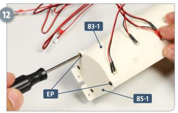
Attach the endplate **85-1** to the deckhead panel **83-1** using two **EP** screws, as pictured.
