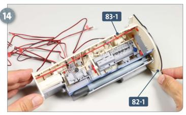
Place the forward bulkhead for the electric motor room **82-1** against the forward end of the deckhead panel **83-1**, so that the two holes of each part are aligned.
