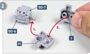
Firstly, fit the peg of the motor housing **H** through the hole in the tab of the cylinder housing **90-6** (arrow 1). Once firmly in place, glue the motor housing I to the other half of **H** (arrow 2).
