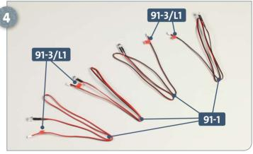
Repeat the process, labelling the remaining three white LED cables 91-1 with a cable label 91-3/L1. Check that all five LED cables work by connecting them to the test board 3-8 (refer to kit 43 for instructions on how to do this if needed).
