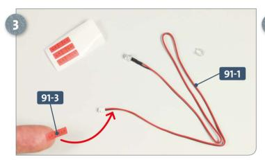
Take one of the white LED cables 91-1 and remove the cable label 91-3 with the label L1 from the backing film. Stick the label to the cable, approximately 8mm from the end with the plug, as shown.
