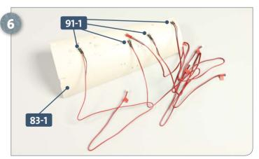
Insert the white LEDs **91-1** into the four other holes in the deckhead panel **83-1**, as pictured.
