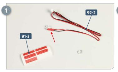
Remove the tie from the red LED cable **92-2** and locate the cable label **91-3**. Note that the red LED has red sleeving (see arrow above).
