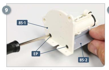
Fix the endplate **85-1** to the ballast tank **85-2**, using two **EP** screws, as pictured.
