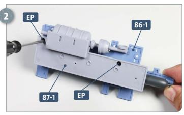
Turn the assembly upside down and attach the base **87-1** to the deck panel **86-1** with the two **EP** screws, as pictured.
