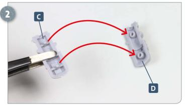
Apply some glue to the two pegs of part **C** and fit them into the corresponding slots in part **D**, as shown by the arrows.
