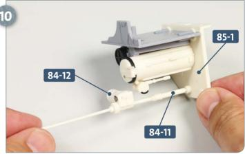
Take the main rudder motor assembly **84-12** that you built in kit 84. Apply a little glue to the end of the drive shaft **84-11** and insert it into the socket in the endplate **85-1**, as shown. If necessary, slightly enlarge the hole in endplate **85-1** with a small pointed file, or similar.
