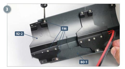
Attach the connector **92-2** to the lower hull section **80-1** using the four **FM** screws.
