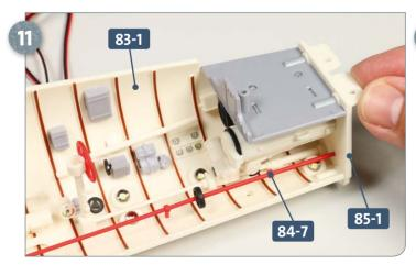
Join the deckhead **83-1** to the endplate **85-1**, making sure that the aft end of the rod **84-7** is inserted into the hole in the endplate. If necessary, enlarge the hole slightly.
