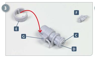
Next glue attachment **G** to the peg of part **D** of the cooling pump. Attachment **E** is then glued to the wider end of the cooling pump, as pictured: the grooves help with correct alignment. See also the photograph in the next step.
