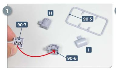
Locate the two halves of the cylinder housing, **90-6** and **90-7**. Apply some glue to the pegs and join the two parts together, as pictured. Detach the two halves of the motor housing, **H** and **I**, from frame **90-5**.
