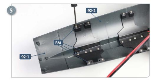
Fasten the hull section **92-1** to the connector **92-2** using four **FM** screws.
