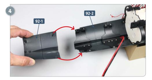
Take the lower hull section 92-1, orient it as shown, and fit its front mounts to the rearmost holes of the connector 92-2, as indicated by the arrows.
