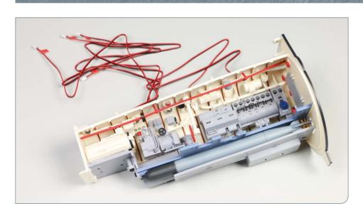
The sixth compartment has now been assembled, with LEDs inserted into the deckhead panel.
