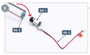
After fitting the cable **96-3** to the circuit board of the motor **96-1**, take the cog **96-2** and fit it onto the hub of the motor **96-1**, as shown.
