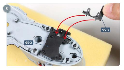
Take the guide **95-3** and insert its two pegs into the holes in the bracket **95-2**, shown by the two arrows.
