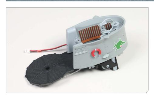
The bearing frame for the direction-finding radio has now been fitted to the upper turret assembly and is connected to a motor.
