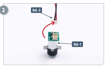
Take the motor **96-1** and connect the terminal of its circuit board to the smaller connector of the cable **96-3**, as shown by the arrow.
