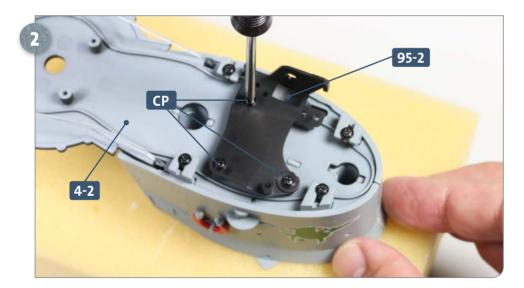
Fix the bracket **95-2** in place using three **CP** screws.
