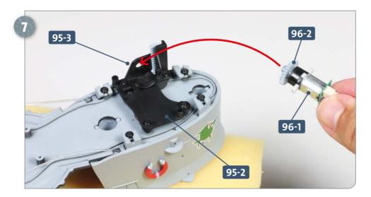
This photo shows the view of the fitted bearing frame for the radio 95-1 from below. If the frame gets stuck when being slotted in, loosen the two screws securing the guide 95-3 and temporarily remove it. Once the frame is inserted, reattach the guide. Next, take the motor assembly and insert the attached cog 96-2 into the large opening in the bracket 95-2, as indicated by the arrow.
