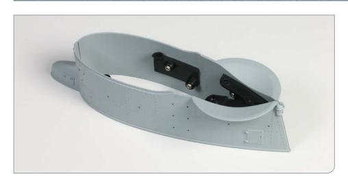
Three connectors have now been attached to the starboard (R) section of the tower, before joining the port (L) and starboard (R) sides together.
