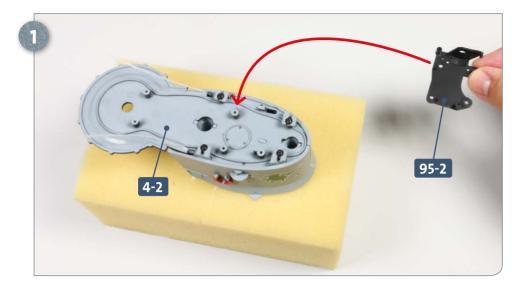
Take the upper turret assembly that you last worked on in kit 5. Carefully turn it upside down, ideally placing it on a soft surface so that the delicate components on top are not damaged. Fit the bracket 95-2 to the three raised sockets in the forward section of the bridge deck 4-2, as indicated by the arrow.
