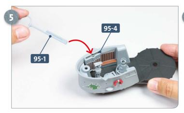
Place the upper turret assembly on your work surface. After noting the orientation of the bearing frame **95-1**, slot it into the opening formed by the fairing part **95-4** and the bulwark. It is important to also see step 7.
