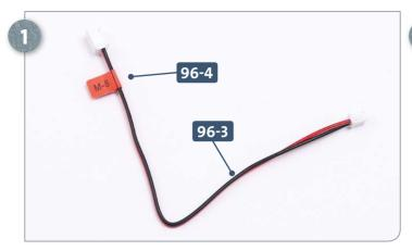
Take the cable **96-3** and cable label **96-4**. Remove the cable label that reads **M-8** from the backing film and attach it to the cable at the end with the larger connector.
