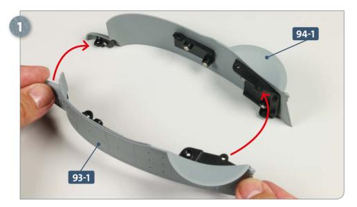
Take the port (L) side of the tower 93-1, which you worked on in the previous kit, and join it to the starboard (R) section 94-1, as indicated by the two arrows.
