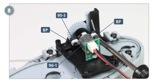
Attach the motor **96-1** to the guide **95-3** with two **BP** screws.
