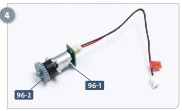
This photo shows the cog 96-2 correctly fitted onto the motor 96-1.
