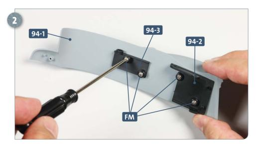
Fix the connector **94-2** in position using two **FM** screws. Next, place connector **94-3** further forward on the tower section **94-1** and fasten it in place using the two remaining **FM** screws.
