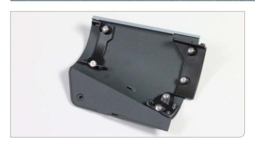
Three connecting parts have now been attached to a portside hull plate.
