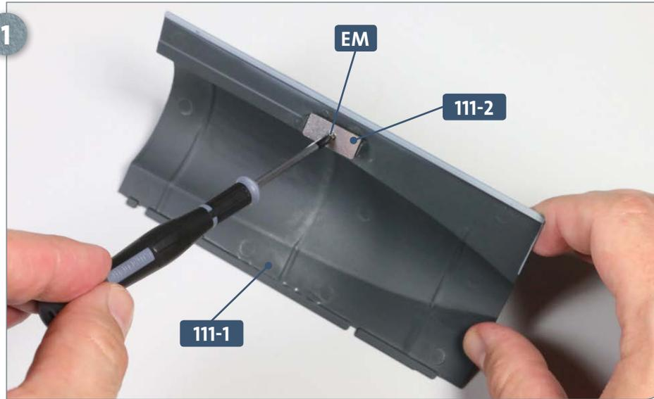
Lay the hull section **111-1** on your work surface with the inner side facing up. Take the metal plate **111-2**, fit it flush with the hole in the hull section and secure it with an **EM** screw, as pictured.
