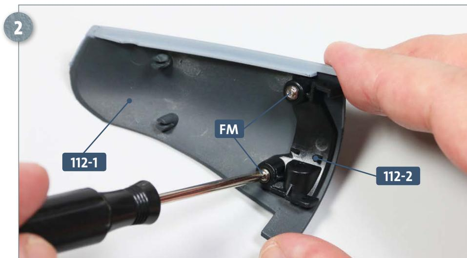
Attach the connector **112-2** in place using two **FM** screws.
