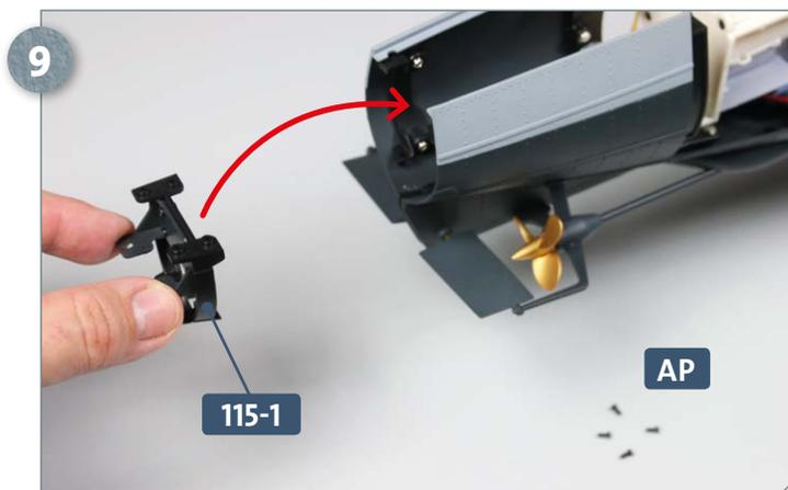
Place your model on your work surface so that you have good access to the aft end. Have ready four **AP** screws. Insert the connector **115-1**, oriented as shown, into the aft of the main structure. See also the next two steps.
