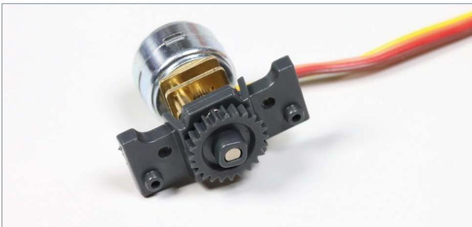
The motor for the rudder has now been fitted with a mounting plate and a cog.
