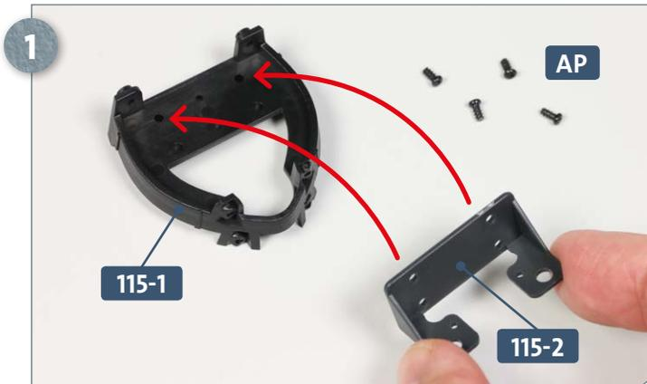
Place the connector **115-1** and four **AP** screws on your work surface. Take the mounting plate **115-2** and fit it onto the connector so that the holes in both pieces align. Also pay close attention to the alignment of the parts themselves.
