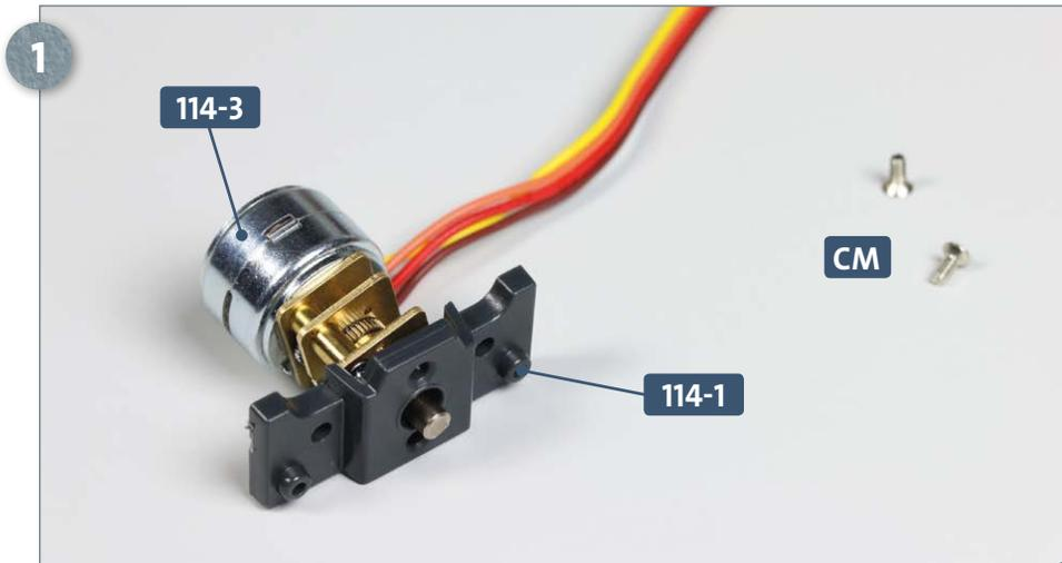
Have ready two **CM** screws. Take the mounting plate **114-1** and fit its hole over the motor shaft **114-3**. Be careful to align it correctly, as pictured.
