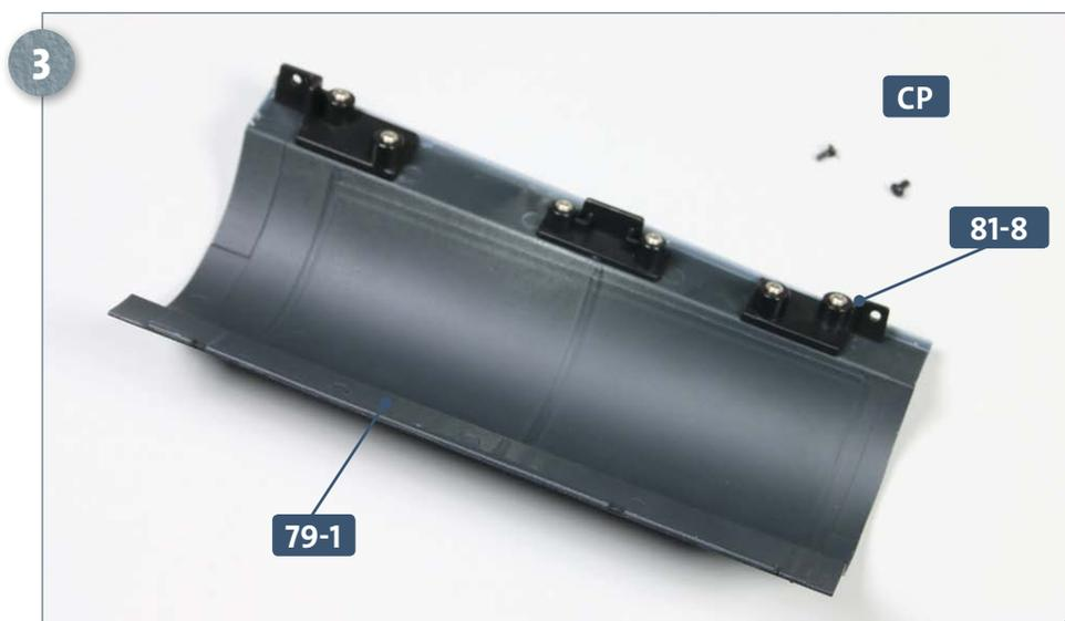
Place the two removed **CP** screws to one side and remove the hull plate **79-1**.
