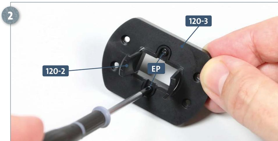
Join the connector **120-2** to the bracket **120-3** using the **EP** screws.
