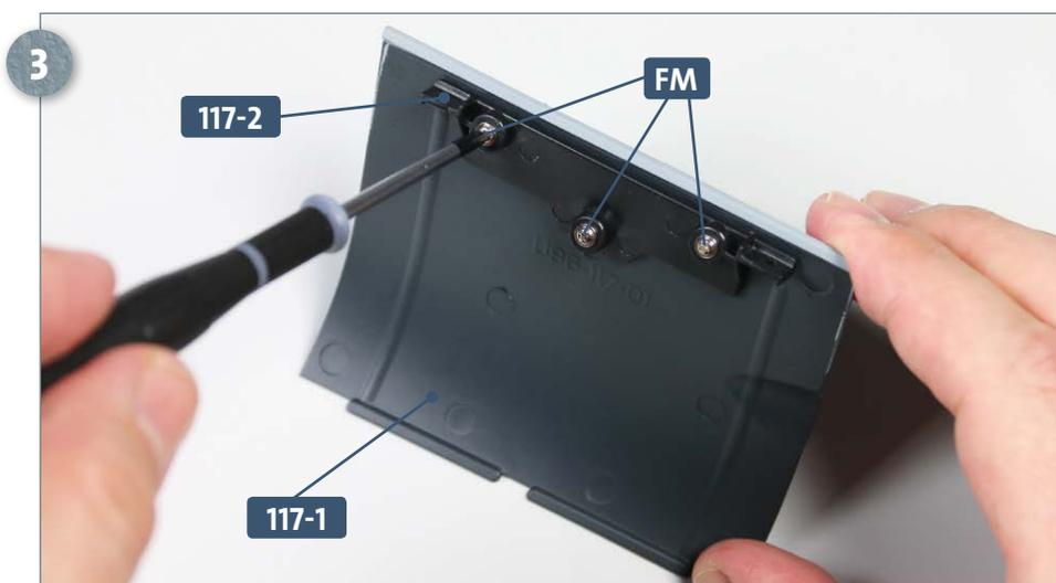
Now fix the connector **117-2** in place with three **FM** screws, as pictured.
